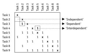
► Figure 3.3 The Design Structure Matrix
