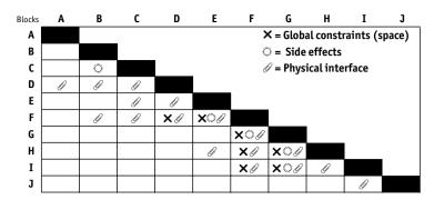
▶ Figure 6.7 The identified physical interactions between the building blocks
