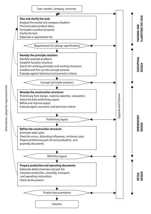
▶ Figure 2.5 Steps in a design process according to Pahl and Beitz
