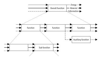
▶ Figure 2.6 Function structure according to Pahl and Beitz
