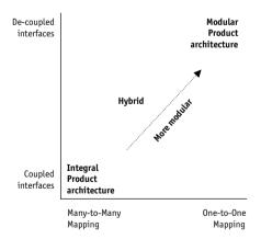
▶ Figure 2.14 The range between modular and integral architectures
