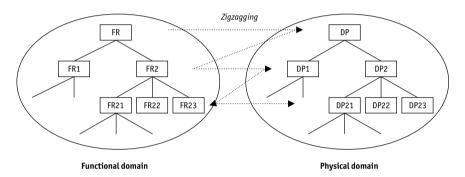
▶ Figure 2.7 Decomposition as zigzagging between the functional and physical domains
