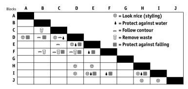
▶ Figure 6.6 The identified mapping interactions between the building blocks
