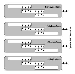
▶ Figure 3.2 Concurrent Engineering in the large for a laptop based on McCord and Eppinger 1993
