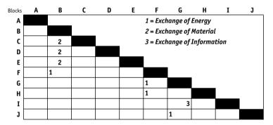
▶ Figure 6.5 The identified functional interactions between the building blocks
